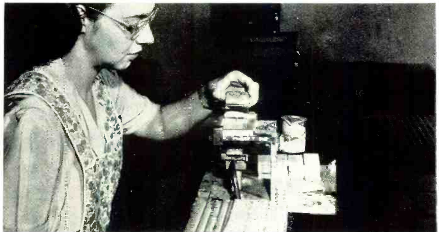
Fig. 4. Silk-screen printing. Paint is forced through the open mesh of the screen. After the screen is removed, the surface of the base plate is found to be printed with an exact, sharp-edged, uniformly-thick design of the required conductor circuit. A second stencil can then be used to print the resistors in their proper location.
